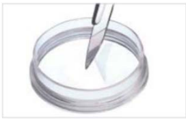
Fig1. shows that the lumox® can be cut out easily and quickly using a scalpel
